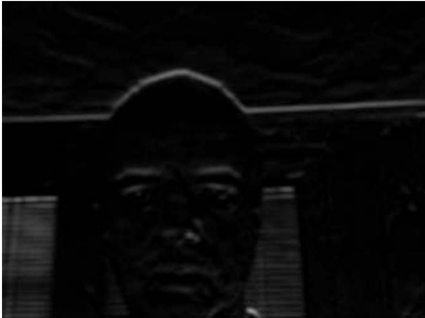
Figure 5-11. Creating horizontal edge detection
