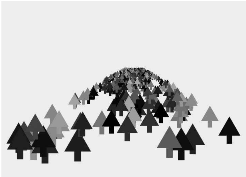
Figure 7-5. Perspective is fine, but no depth sorting
